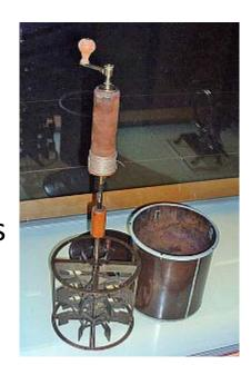
Joule used this apparatus to make the fundamental connection between heat and work. Picture from Wikimedia C
