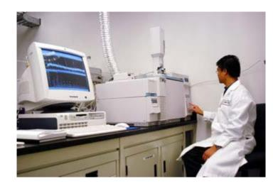
Environmental chemists frequently use <u>GC-MS</u> to analyze samples. The technique can detect very low concentrations of pollutants.
